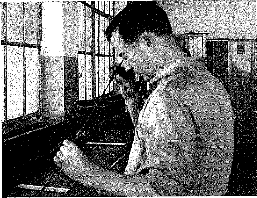
Inspecting pinion rod prior to shipment.
